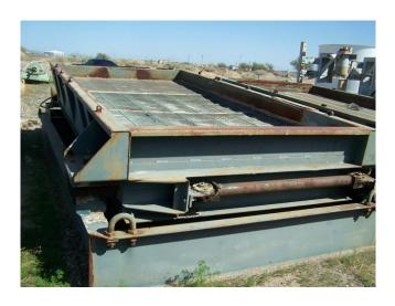
Used Rotex Screen. Model: 7221 10 HP Motor. Supplied with Extra SS Screen Cloths.
