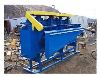
Bank of 4 Denver #12 DR Flotation cells. Units supplied refurbished and shipped to Northern Canada.
