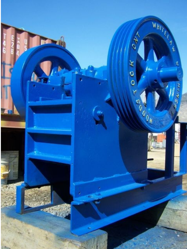
Whitelaw 5in. X 12in. jaw crusher. Comes with near new liners and cheek plates.
