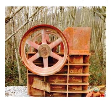
Used Hewitt Robins Style Jaw Crusher. 24 in. x 36 in. Custom Built Stand. 125 HP Electric Motor. Extra set of Jaw Plates.
