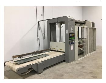
Model: CF-2000Horsepower: 3 HPVoltage: 480 Volt
