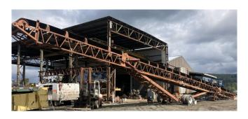
Portec 36in x 105ft Radial Stacking Conveyor
