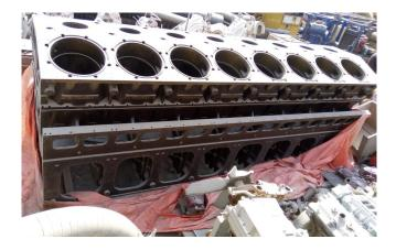
MWM Deutz 16 Cylinder 640 Series Crankshaft and Block
