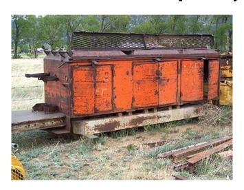
Maintenance/utility car. 16 feet long X 4 feet wide. On 24 in. track guage. Comes with 2 open compartments and 1 multible shelved compartment. All with hinged front doors.
