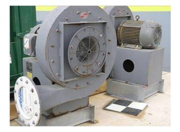
Hartzell high pressure blowers. Model 07T-235-PBS2. 4261 CFM SP(in W.C.) 36. Driven by a 40hp 230/460 volt 3450 rpm motor. Located in San Atonio, Texas.
