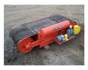
Eriez 44in wide X 9.5ft long cross belt magnet. 3hp belt drive motor. SOLD. SUPPLIED REFURBISHED AND READY TO INSTALL.
