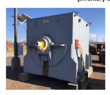
Electric Machinery 8,000HP Squirrel-Cage Induction Motor
