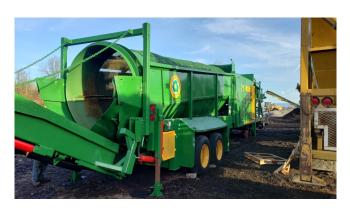
The 621 Trommel is a proven reliable machine in construction and demolition, topsoil, compost, waste recycling, and many other large screen applications. Powered by 174 HP engine suited for large heavy duty applications where production rates can reach 200 + TPH in topsoil and sticky material or 300 + TPH in sand and gravel.
