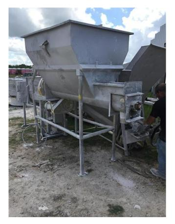
Rietz 50ft<sup>3</sup> Stainless Hopper with Auger Discharge
