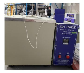
Asian Test Equipment Heat Deflection Temperature Tester
